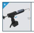
Hold the sealant gun upwards so that the two components come out of the mixing nozzle simultaneously. Discard the first material to come out that is not
