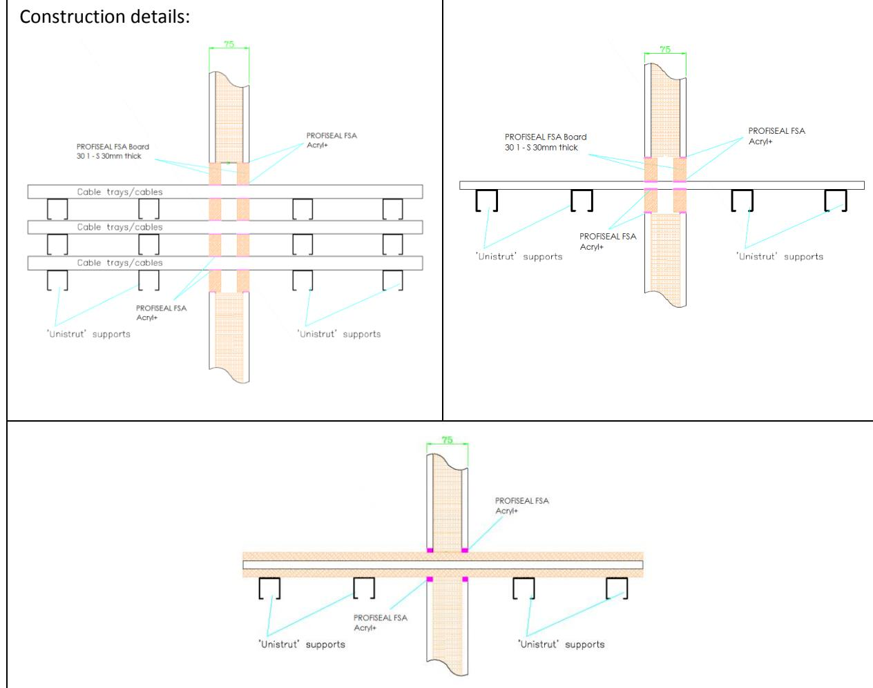
**A.3.1.1 Double side penetration seal with cables**
