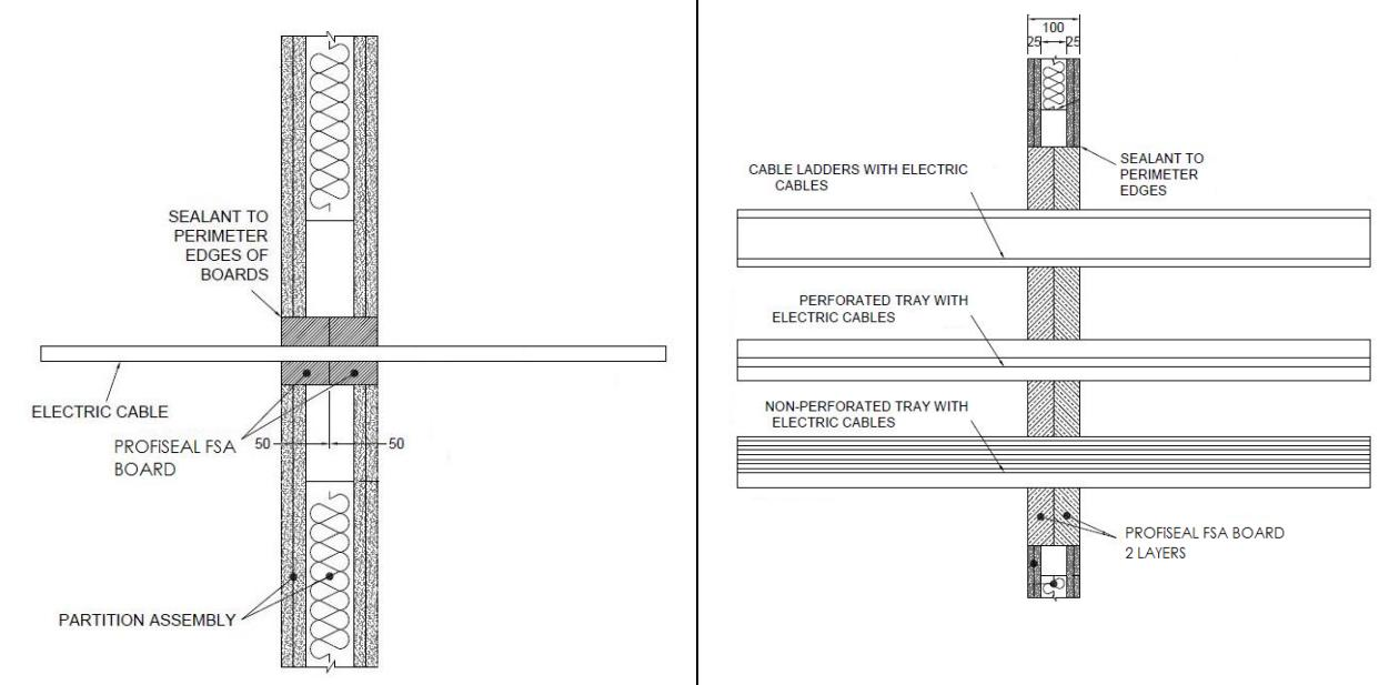
Note: Insulated metal pipes may also be included within the same seal as cables subject to minimum 100 mm separation. See separate classification for pipes.
