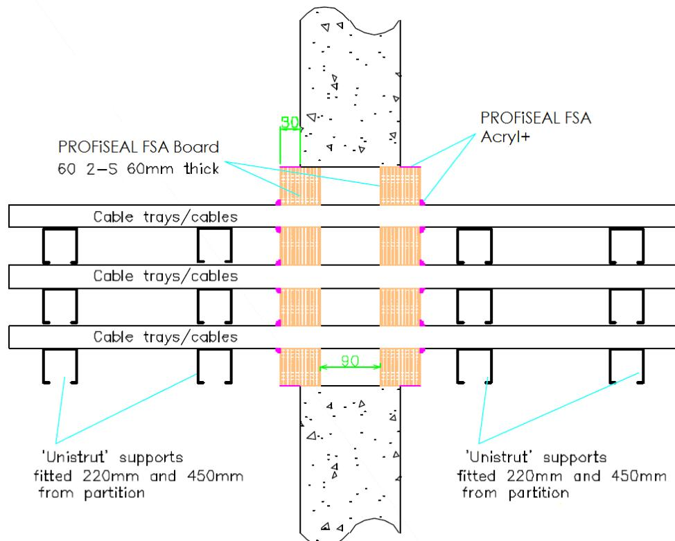
**A.1.6.1 Two side penetration seal with cables**
