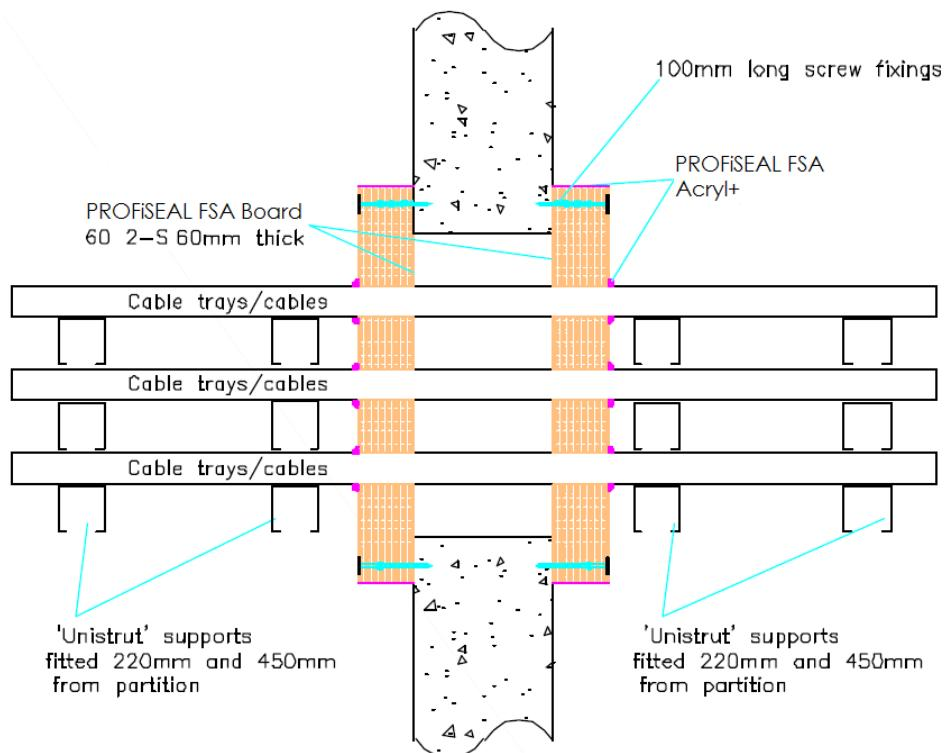
**A.1.7.1 Two side penetration seal with cables**
